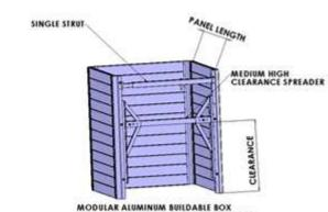
MODULAR ALUMINUM BUILDABLE BOX WITH MEDIUM HIGH CLEARANCE SPREADER
