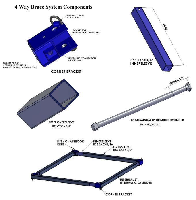
HYDRAULIC BRACE FRAME ASSEMBLED
